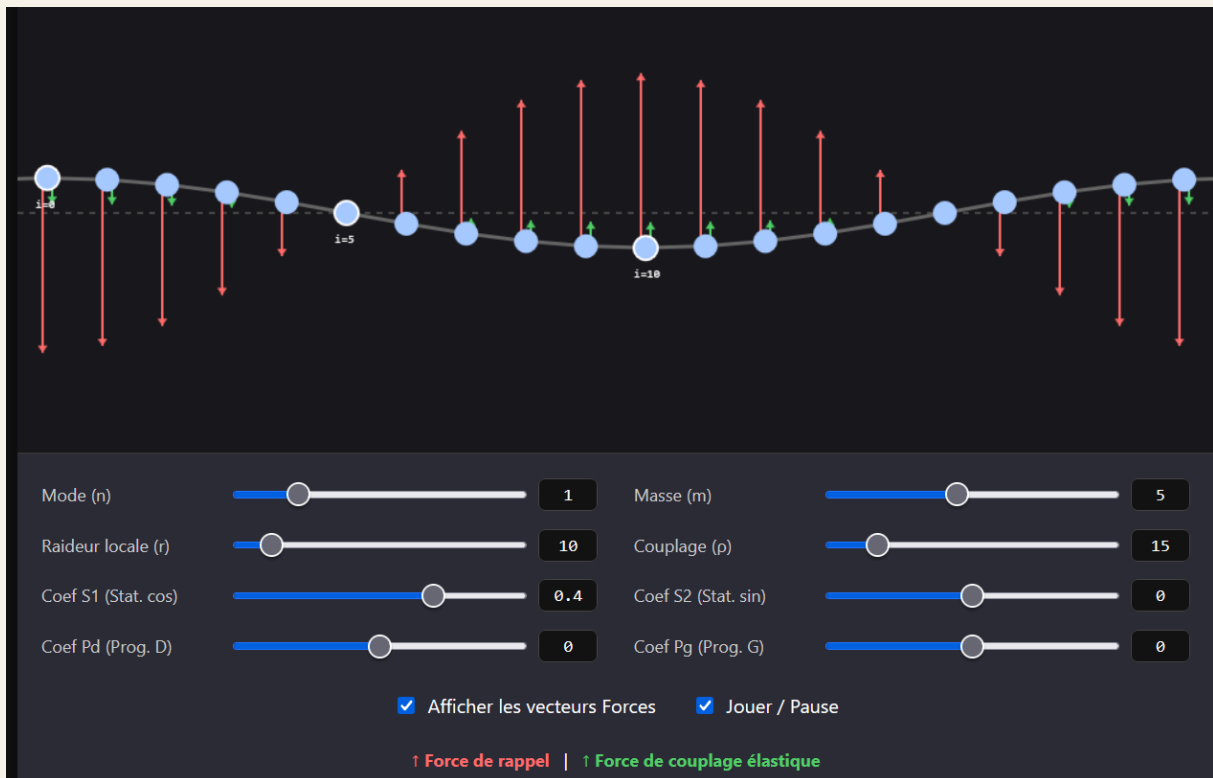
Figure 17: mode 1. The elastic coupling force is present but remains weak, so the frequency increases only slightly.
