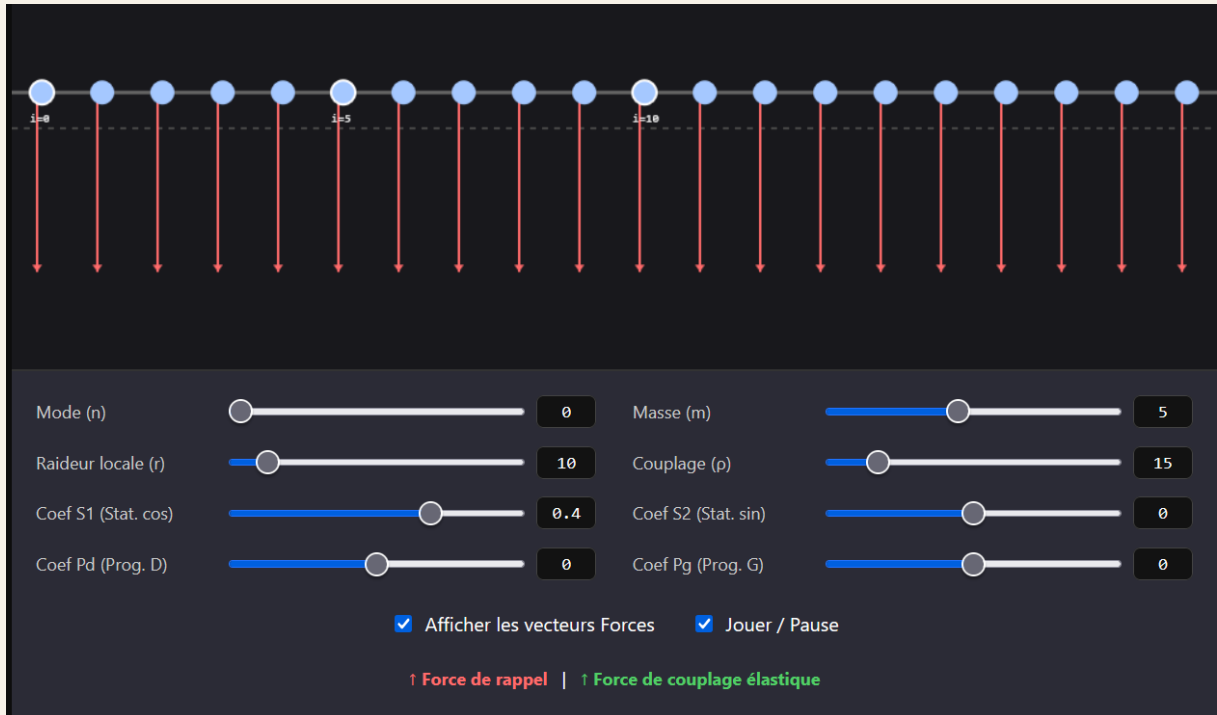
Figure 16: fundamental mode n = 0 . The elastic coupling force vanishes, so the effective restoring force on each mass, and therefore the frequency, is minimal.
